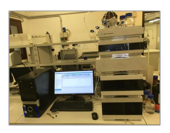
The Agilent 1290 Infinity LC is an UHPLC (Ultra-High Performance Liquid Chromatograph) equipped with binary pump, diode array detector (DAD), column heater and autosampler. This LC system performs analyses with high chromatographic performance and resolution, combining ultra high pressure up to 1200 bar and high flow rates up to 5 mL/min.
