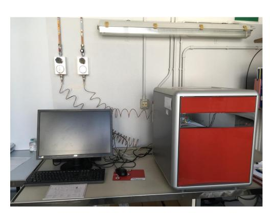
The vario Micro cube is an innovative elemental analyzer for C,H,N,S and halogens determinations. This instrument incorporates a newly developed gas separation method: gas are sequentially separated by a temperature programmable desorption column (TDP) and quantitatively determined on a thermo-conductivity detector.
