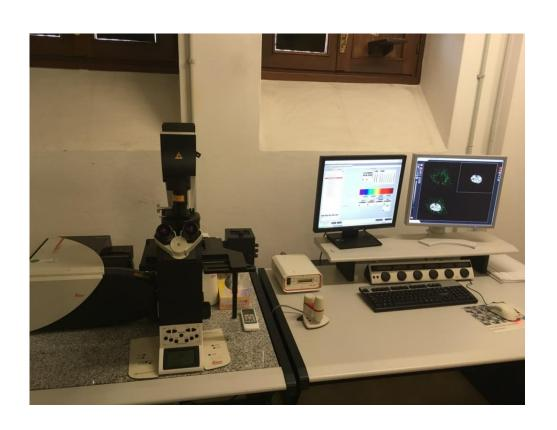
The Leica SP5 is a flexible, fully-featured laser scanning confocal microscope suitable for high resolution imaging of fixed and live samples. It provides a spectral range from UV to IR and it allows the investigators to use a large variety of fluorescent probes. It has an inverted DMI6000B microscope stand capable of fluorescence.
